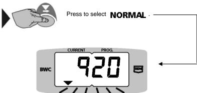
The left-hand section shows the current number of wraps and the right hand section shows the target number. When the current number = Target number, the alarm will sound for 2 seconds and the display will flash. (If set, the early warning alarm sounds beforehand).
